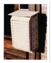
Ordinary spirit-in-glass thermometer. This simple louvred thermometer screen is available as a kit
