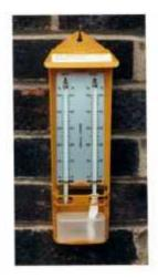
Humidity is measured most accurately with a wet- and dry- bulb thermometer
