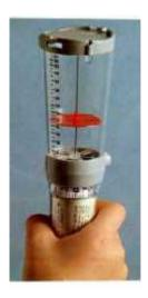
A simple home-made weather-vane The ventimeter can measure wind speed and indicate wind direction
