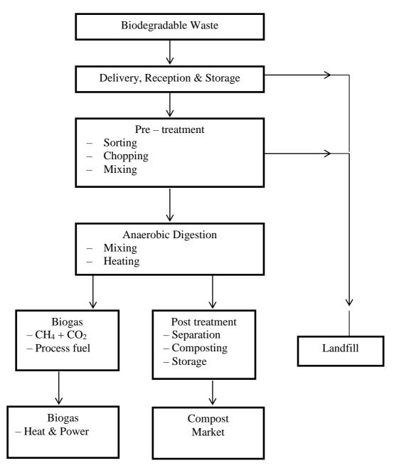
Fig 2. Schematic diagram of the anaerobic digestion process for biodegradable waste. Sources: McLanaghan 2002; IEA Bioenergy 1996.
