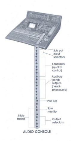
**Mix:** The audio console enables one to combine, or mix, the signals from various inputs, such as two lavaliere mics, background music, and the sound effect of a phone ring. The mix bus combines (mixes) these various audio signals with the specific volume assigned by the operators. Without the mixing capability of the board, one could control only one input at a time. The completed mix is then fed to the line-out.
