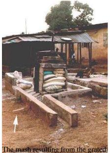
The mash resulting from the grated roots are squeezed free of liquor in a press. To eliminate the nuisance the liquor is led by a pipe (arrow) into a 23 pit
