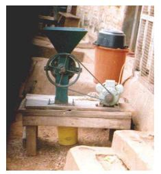
Peeled roots are grated in mechanical arrangements
