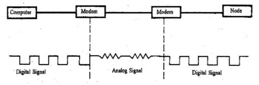
Figure 3: Signal conversion by modems i.e Modulation and Demodulation
