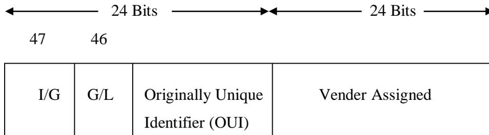
Fig. 4.4.1 – Ethernet addressing using MAC addresses
