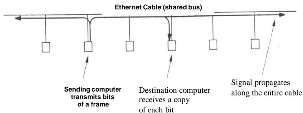
Fig. 2.2.1 - Conceptual flow of bits across an Ethernet
