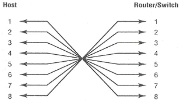
Fig. 4.3.8 Rolled cable
