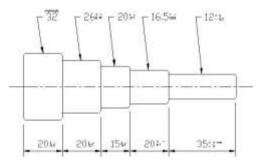
9. Face off the remaining material, so that the 12 diameter is left at 35 long (+ or - 0.5 mm).
