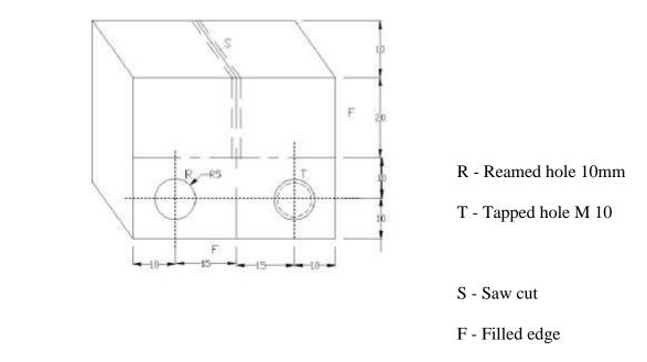
To drill, file, as shown in the sketch, ream and tap holes on the mild steel plate.
