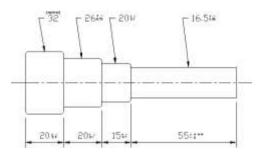
8. Turn the 12 mm diameter x at least 35 mm long - ensure that the diameter is left at 12 mm + 0.0 and -0.1 x 35 mm long. (see the diagram below).
