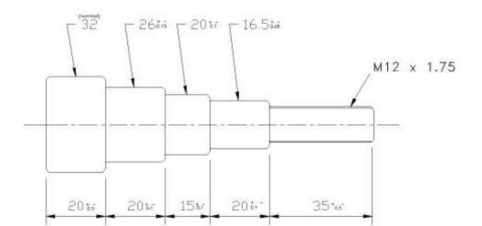
6. Turn the 20 mm diameter x at least 70 mm long - ensure that the diameter is left at 20 mm + or  $-0.1 \times 15$  long. (See the diagram below).
