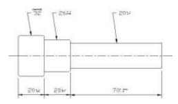
7. Turn the 16.5 mm diameter x at least 55 mm long - ensure that the diameter is left at 16.5 mm + or -0.05 x 20 mm long. (see the diagram below).
