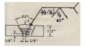
**Observation:** After cooling and chipping the slag off, inspect the beads for width, build up, molten weld pool size, spatter, and penetration. Record your observations on a <u>Student Welding Report.</u>
