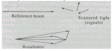
Addition of a strong coherent reference beam (top left) with random-phase signals (top right) gives similar resultant (bottom)
